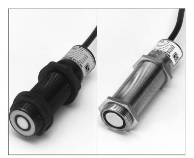
The RPS-401 housing is constructed of PVC plastic and the RPS-426 is Stainless Steel. The housing is 30mm in diameter by 100mm in length. For set up purposes an LED indicator is provided. The LED will illuminate green when nothing is detected and will illuminate red when a target is detected. A standard 6' cable is provided or a quick disconnect (QD) version is also available.
